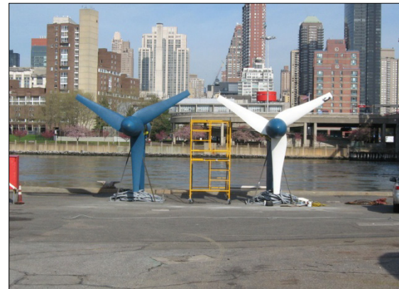
Figure 6 - Verdant Power's Free Flow Kinetic Hydropower System Turbines on the shore of their deployment site in New York City's East River.
