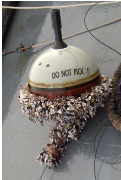
1 2 3 Figure 3.6.1-1. Growth of biofouling organisms on a floating spherical buoy after 521 4 days at sea. Source: National Oceanic and Atmospheric Administration 5 http://www.aoml.noaa.gov/phod/dac/gdp_drifter.html 6 7
